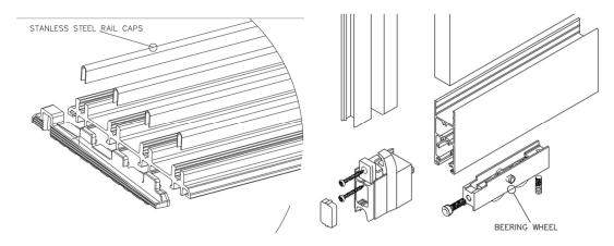
One bearing wheel durable against 150 kg load and two pieces use at each panel. Maximum panel would be 1.20X3.00 meter at DELUXE XL and total weight of such a panel is 90 kg. Against 90 kg max load, the wheels at DELUXE XL durable against 300 kg load.
