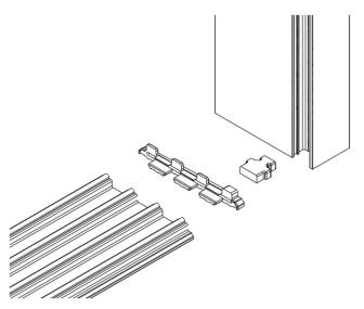
With corner conjunction kit, we are adding additional drainage against rain or snow waters. Thus water will not accumulate at corner parts and directly flow the outside area.
