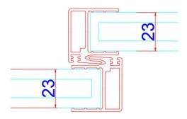
As shown at above picture, connection between two panels provided with carrier profile and against wind, dust and water, it is strengthen with brush seals which is placed two sides of connection parts.
